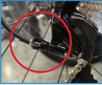
To adjust the rear mech/derailleur, screw the barrel adjuster on the end of the cable housing.
