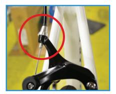
The barrel adjuster is situated at the top of the brake caliper, screw the adjuster to tighten the cable.
